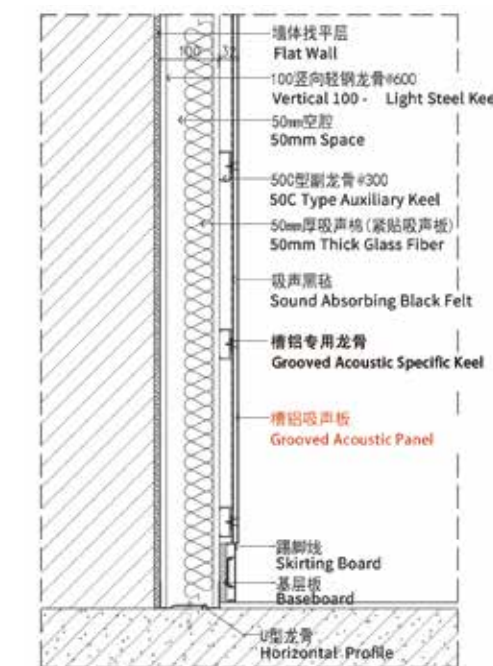
槽铝吸声板墙面安装竖剖图 Vertical Section Of Grooved Acoustic Panel Wall Installation
